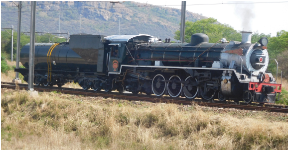
Steam hauled out of Pretoria behind engine number 3360, a 1949 North British build class 19D (Note the extra large water tender to cope with going across the arid Karoo desert)
