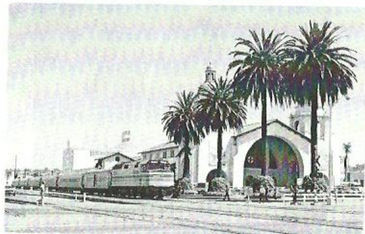
SAN DIEGAN Amtrak's morning train from Los Angeles arrives San Diego at the mission style station. Passengers now enjoy the new Amfleet cars placed in service only a few months before this August 1976 scene. Power, including heating, lighting and cooling needs, for these new trains is supplied by General Motors F40PH, 3000hp locomotives
